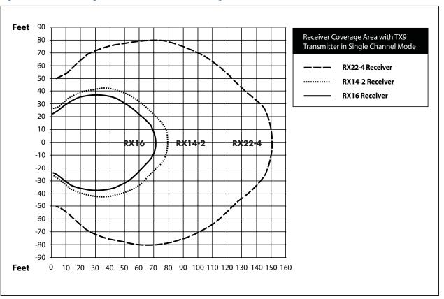
The coverage area for the TX9 will vary depending on the receiver being used. The diagram above demonstrates the receiver coverage when operating a single TX9 emitter in single channel mode. Patterns are direct radiation patterns.
